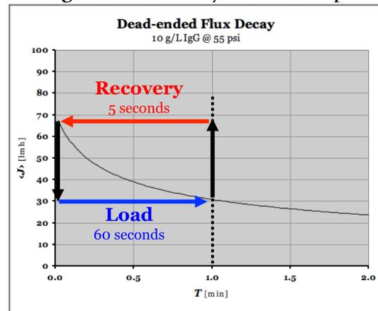
As expected, the instantaneous flux during the loading step decreases with time. However, once the boundary layer is removed, the flux recovers fully for the next cycle, delivering a high average stable flux for the duration of the process.
